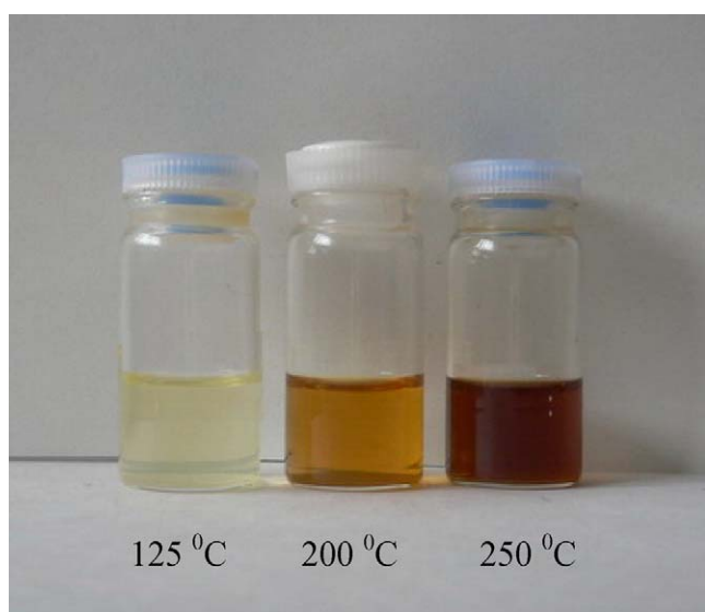
Fig. 2. Soluble reaction product obtained at 125, 200, and 250 °C after 10 min.
